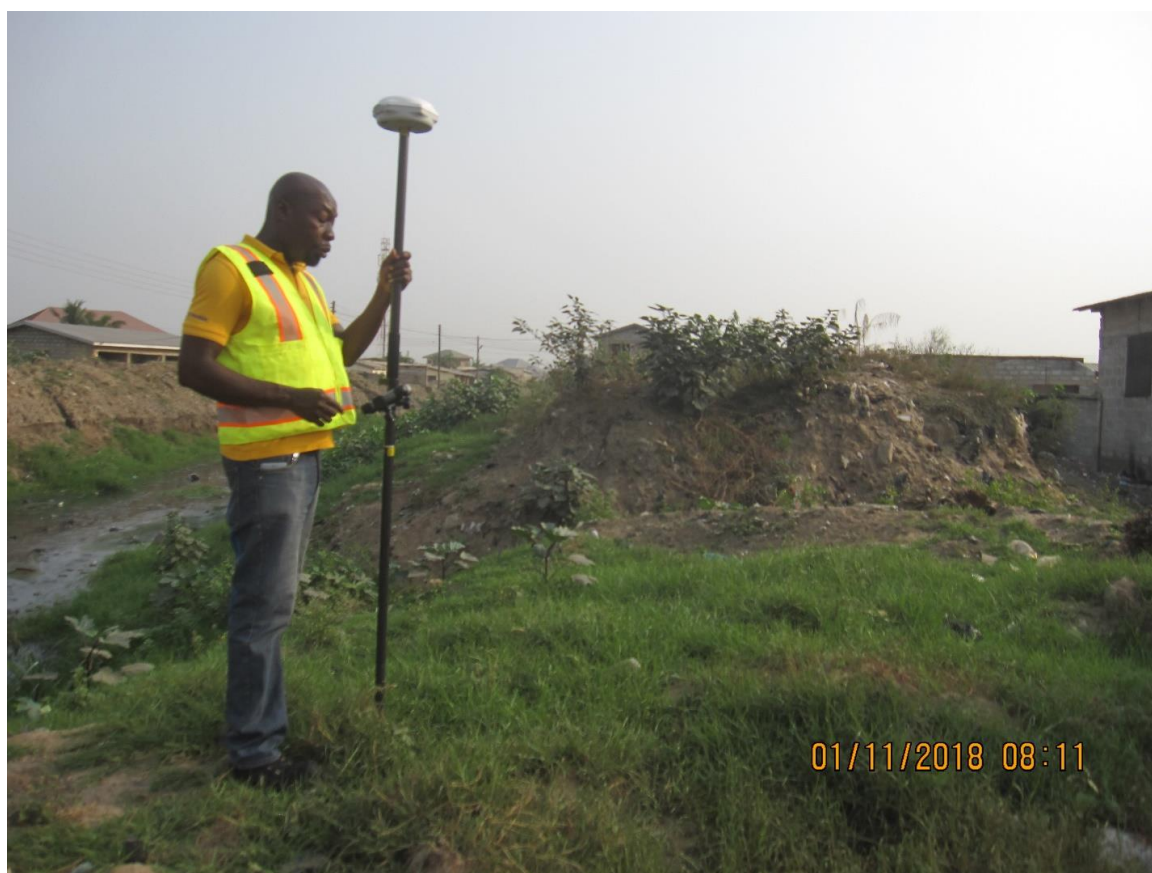
Figure 3.1 Rover receiver capturing data along the proposed trunk sewer route
