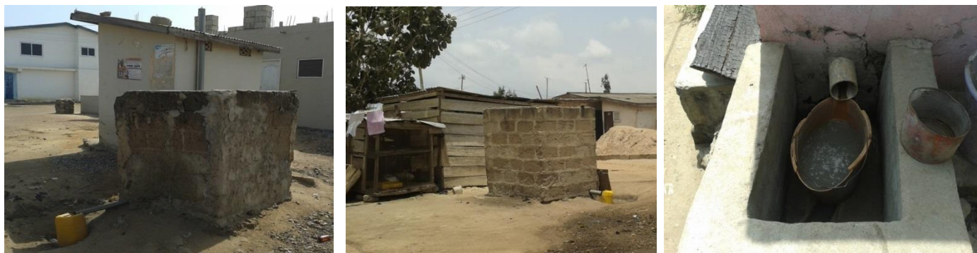
Plate 4.11: Use of gallons and buckets as bathroom wastewater collection containers
