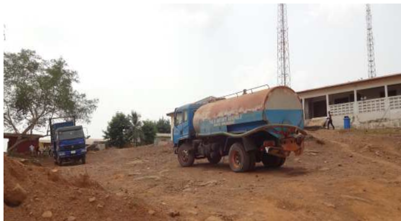
Plate 4.2: Cesspit Emptier (vacuum suction) truck owned by the Twifo Hemang Lower Denkyira District Assembly.
