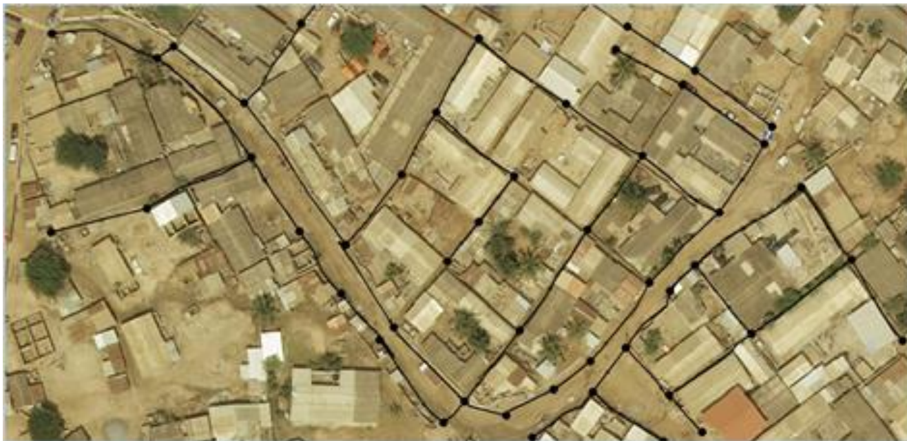
Figure 3-7: Layout of block sewers for simplified sewer network in Teshie Old Town showing congested (dense and interlocked) nature of houses
